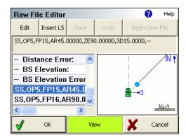
Perpendicular Offsets - point picker is a check-box type button and will now remain in effect until switched off.
